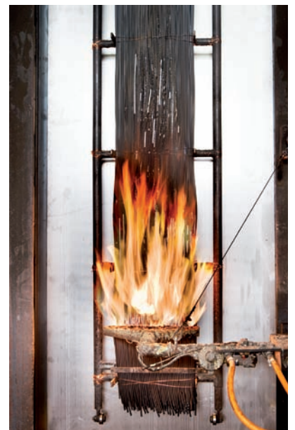
Image: Flame propagation test on a cable bundle
